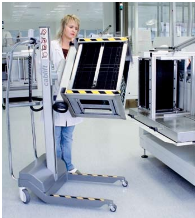
The Minilift as a flexible magazine-loader
